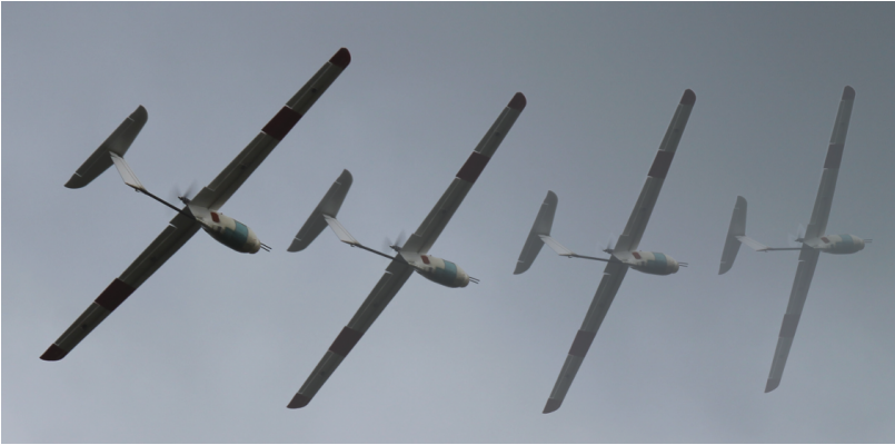
Figure 7.1: Techpod, fixed-wing unmanned aerial test platform.
